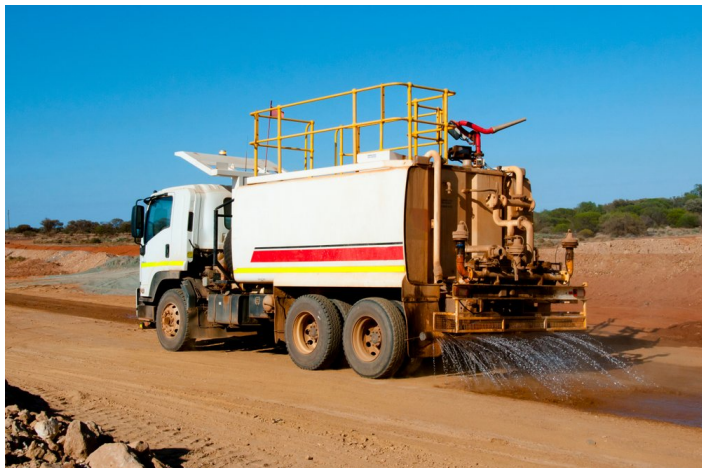
Water carts will be used to mitigate dust.
