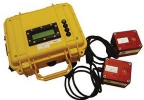
Vibration monitoring device.
