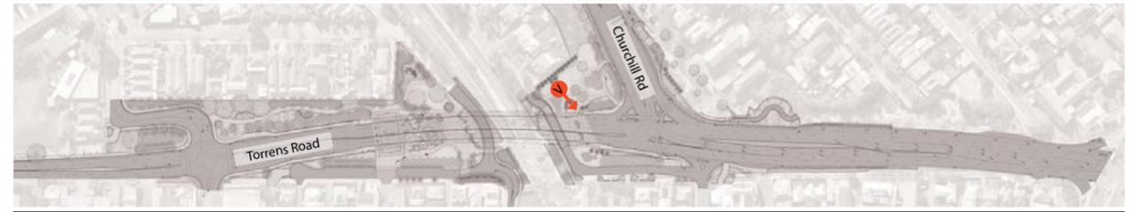
To meet traffic sight line requirements, the bridge deck and barriers are required to splay outwards at the north-east corner.
